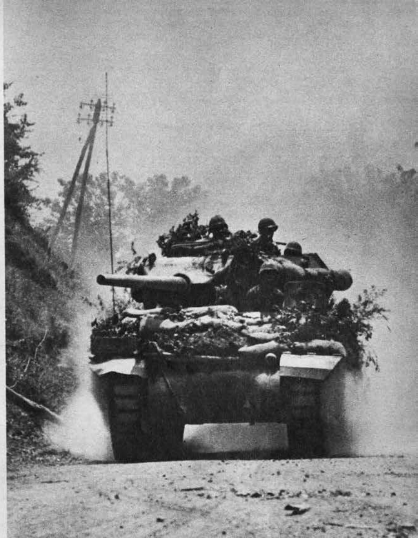
M-10 ANTITANK GUN HAS MEDIUM TANK CHASSIS, OPEN-TOPPED TURRET
